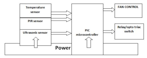
Figure 1: Block Diagram of The System
