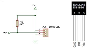
Figure 5: Design of Ds1820 Temperature Sensor
