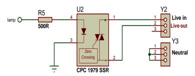
Figure 4: Light Control Using Solid State Relay
