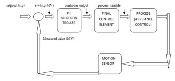
Figure 2: Typical Control Loop of System Performance
