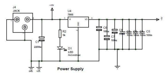
Figure 12: Power Supply Circuit Design
