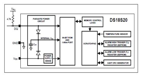
Figure 6: Internal Structure of Ds1820
