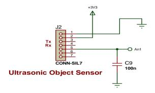
Figure 10: Pin Diagram of the Ultrasonic Sensor
